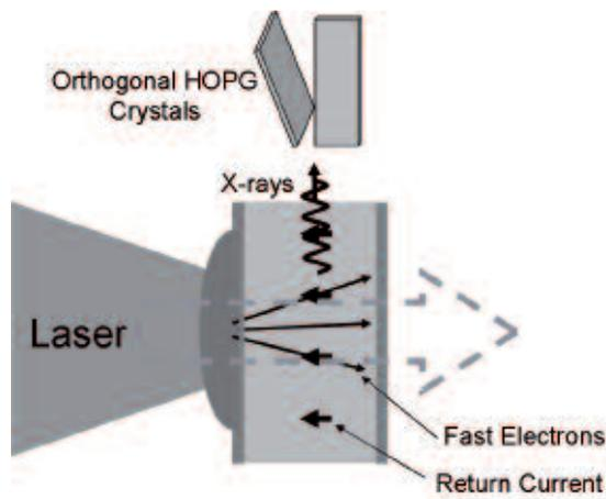
Figure 2. Schematic diagram of the experimental layout, include fast electron generation and return current heating within the target.
