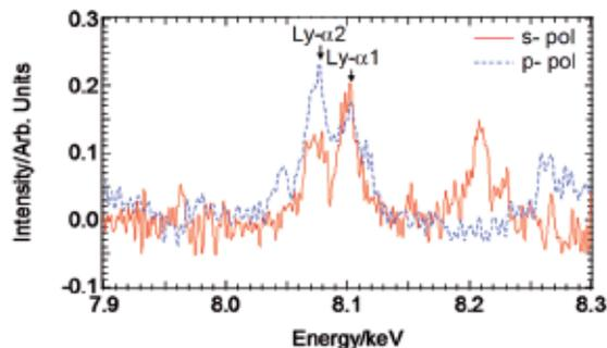
Figure 5. Lineouts of HOPG spectrometer images recorded from a Ni foil target with no tamping irradiated by  $I \approx 10^{21} \text{ Wcm}^{-2}$ .
