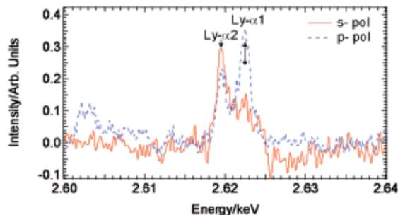
Figure 4. Lineouts of the HOPG spectrometer images recorded from a PS foil target with  $0.2 \mu\text{m}$  Al tamping on the front surface irradiated by  $I \approx 10^{19} \text{ Wcm}^{-2}$ .
